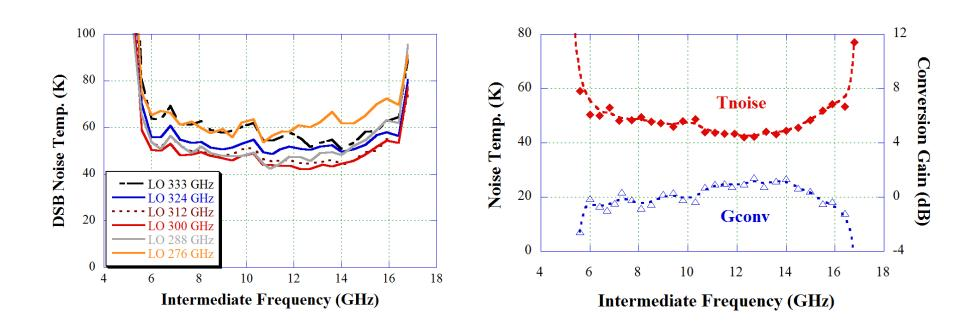
Following upgrades to 1.3 mm receivers, need to do the same with 0.86 mm receivers New 0.86 mm receiver has low-noise across a 6-16 GHz IF compared to 4-8 previously In addition, the noise at the band edges 260, 350 GHz is as low as at band center previously However, need to work towards extending IF down to 4 GHz Expect installation of new receivers to begin early 2013
