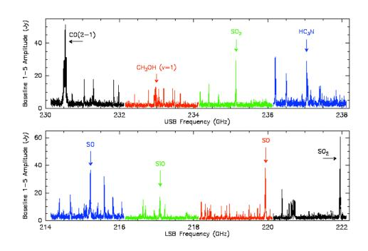
On-sky test observations towards Orion BN/KL on a single baseline: The black spectra show the original 4 – 6 GHz spectral region. The red spectra show the additional coverage obtained in the 'Bandwidth Doubled' mode of operation introduced in 2010, with the usual 12 GHz LO sent to the Bandwidth Doubler Assembly.
