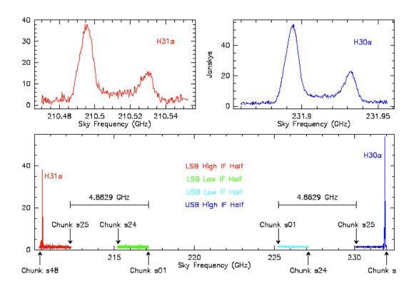
Because changing the LO to the Bandwidth Doubler Assembly allows the two halves of a sideband to span as much as 8 GHz, which is also the separation between the lowest USB frequency and the highest LSB frequency, one can now target any two spectral lines which are separated by less than 24 GHz, either by putting them both in one sideband, which offers coverage for up to 8 GHz separation, or by putting them in different sidebands for up to 24 GHz separation.
