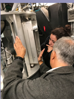
Ram Rao (left) showing the students the inner workings of the SMA antenna, and how the optics direct the light coming from the sky to the receivers in the cryostat below.
