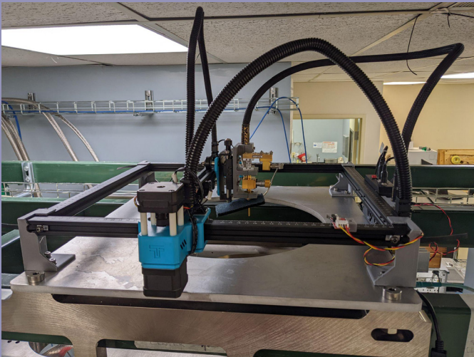
Figure 1: Millimeter-wave beam scanner based on a laser engraver system installed on top of the “Proto-1” wSMA receiver system. The gold colored millimeter-wave source hardware has been mounted in place of the engraver’s diode laser module.
