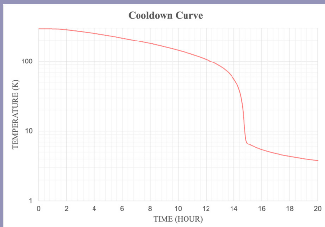
Figure 1: Temperature of a receiver cartridge measured during cooldown of the new wSMA cryostat. A base temperature of 3.5 K was reached 20 hours after the compressor was turned on. At the 18 hour mark, the temperature fell below 4.2 K, the normal maximum operating temperature for SIS mixers.
