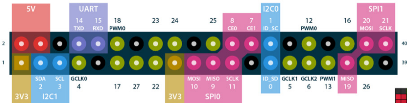
Figure 1. The top image shows the most recent version of the Raspberry Pi single board computer, version 3 model B+. The CPU used is the BCM2837B0, Cortex-A53 (ARMv8) 64-bit SoC @ 1.4GHz. The bottom image shows the pin layout and numbering scheme. For more information, see https://www.raspberrypi.org/products/raspberry-pi-3-model-b-plus/ and https://pinout.xyz/pinout/ .
