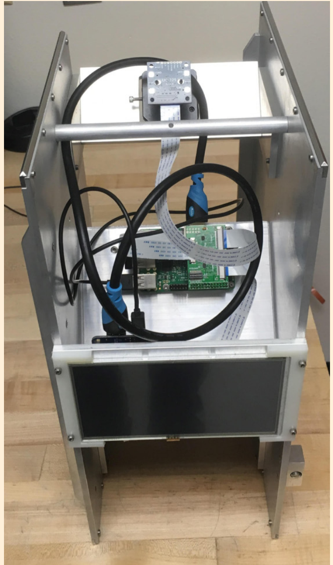
Figure 2. The above figure shows the reference optics insert with the integrated Raspberry Pi and dual camera setup. Since this is powered with a USB power bank, it can be used as a stand-alone unit. This unit was developed by Lingzhen Zeng.
