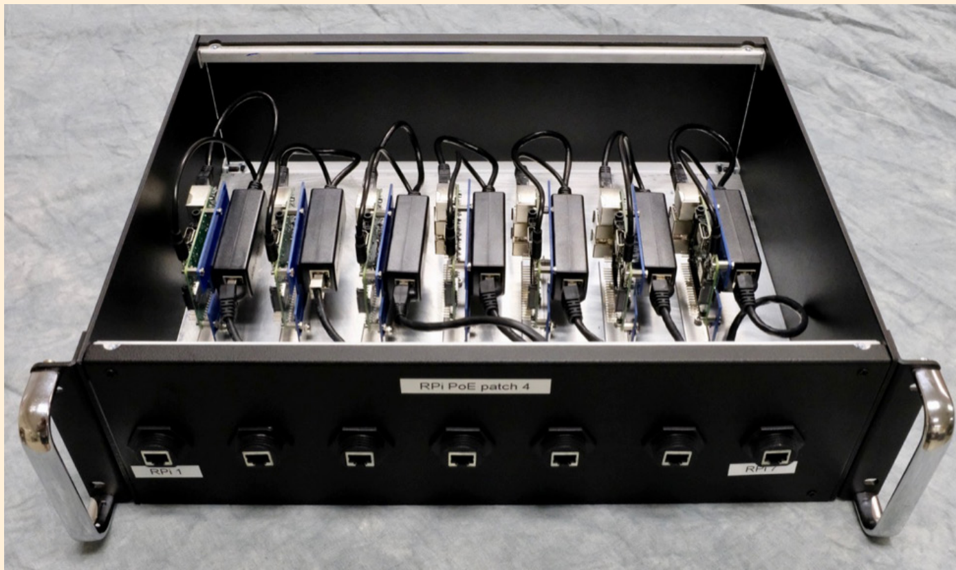
Figure 3. The above figure shows the most recent version of the Raspberry Pi Patch. This features 7 Pis with separate external ethernet ports which can be used also as Power Over Ethernet (POE). (Photo credit: Steve Leiker).
