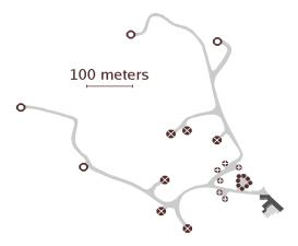
Fig. 1. The SMA antennas are usually configured in one of four approximately circular rings, with maximum baseline lengths of 25 to 508 m, offering angular resolutions of 5 to 0.25 arc-seconds at 350 GHz, the optimal frequency of the array for continuum sensitivity.
