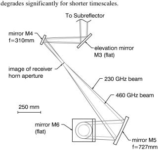
Fig. 4. The SMA antenna beam waveguide assembly used to couple radiation from the antenna to the receivers produces a compact image of the feed between the two ellipsoidal mirrors and provides a convenient location for receiver gain calibration and for the quarter wave plates required to enable polarimetry observations.
