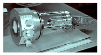
Fig. 5. Photograph of a 650 GHz receiver insert showing, from left to right, the vacuum window, electrical connectors, radial o-ring seal, interface to the 70 K radiation shield, mixer feed with Teflon dust cover. Further to the right: IF isolator and 4 - 6 GHz preamplifier.
