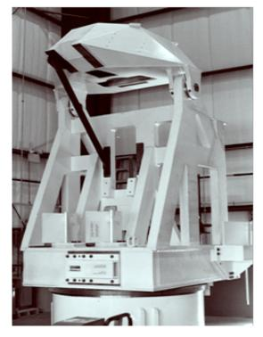
Fig. 2. Photograph of the SMA antenna pedestal. The structure above the elevation bearings connects to the reflector assembly.
