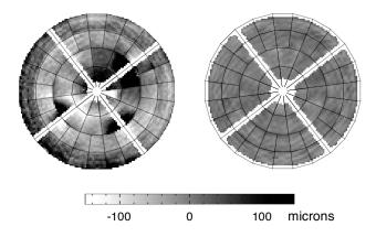
Fig. 3. The SMA antenna reflectors are typically set to  $60 \ \mu m \ rms$  (left) using a mechanical swing arm. A near-field holographic technique, using a phase-locked beacon at 232.4 GHz, is then used to progressively improve the surface. Three iterations are generally required to reach the design specification of 12  $\mu m \ rms$  (right).
