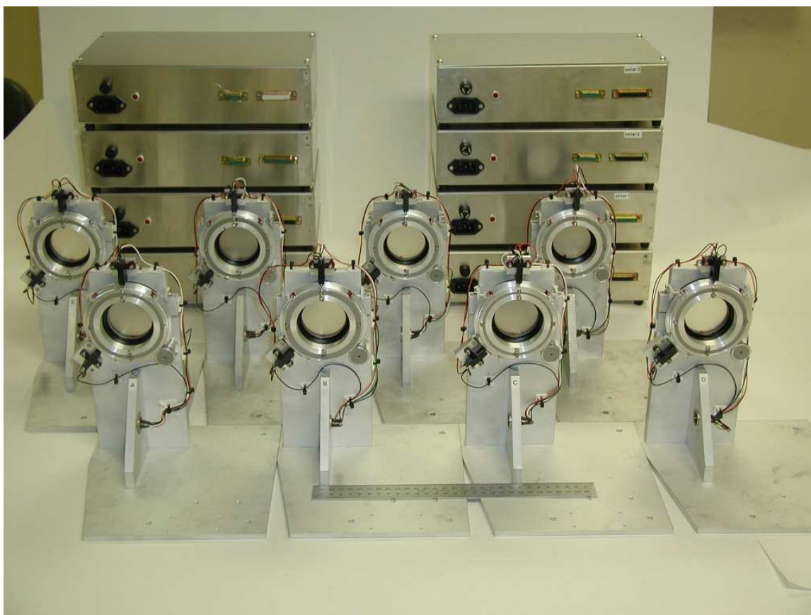
Fig. 2.5.— The SMA wave plate positioning system. The eight wave plates and their positioning stages are in the foreground. See the rotation stage detail in Figure 2.6. The control computers and associated electrical components are in the enclosures at the back. The ruler in the foreground is 30 cm long.
