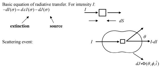
Extinction completely described microscopically by absorption plus scattering.
