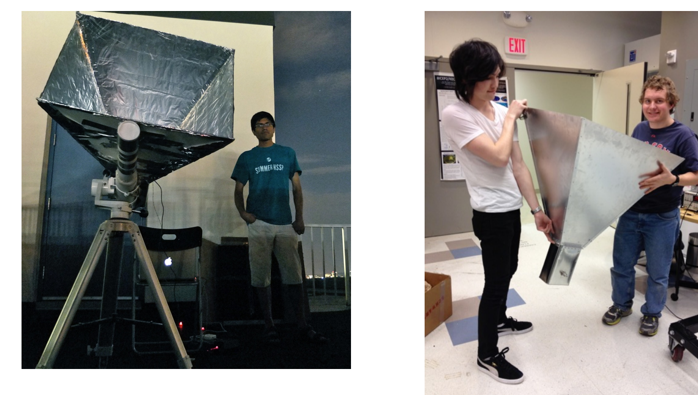
Fig. 5: Left: Cardboard+Al foil horn antenna mounted on a standard alt-az telescope mount in an urban environment. HI spectra toward the Galactic plane are easily detected in just 30 seconds of integration with the system described here. Right: Horn of same dimensions made with aluminum sheet metal riveted at edges. This horn is also light enough to be mounted on standard amateur telescope mounts.
